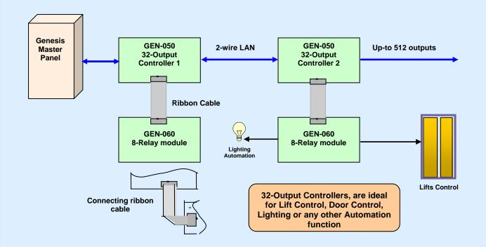
Up to 4 relay modules are supported on the Genesis GEN-050 32-Output controller
