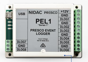
104mm x 72mm x 27mm 150g 12 Volt D.C. operation (10 - 15 Volts D.C.) Operating Temperature: 0°C to 50°C
