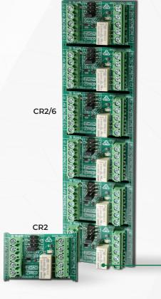
12 or 24 Volt D.C. operation (10 - 18V V Link ON), Maximum Switch Current: 2A at 30V +TR Trigger: 2 to +V, 1.2mA @ 12V, 2.4ma @ 24V -TR Trigger: 0 to (+V-2V) -1.2mA @ 12V, -2.4ma @ 24V \* all voltages D.C. Single unit: 50mm x 31mm x 15mm Strip of 6: 50mm x 186mm x 15mm
