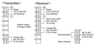
\*Relay shown in energised (non-alarm) condition
