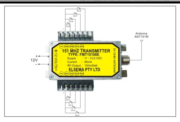
Inputs of the transmitter should be voltage free contact closure only.
