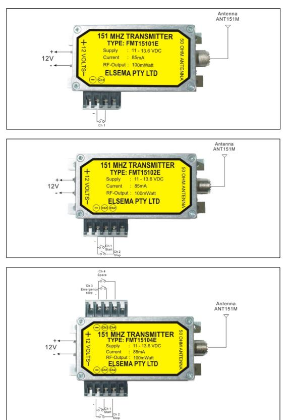
Inputs of the transmitter should be voltage free contact closure only.
