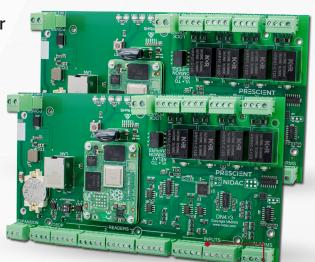
195mm x 107mm x 31mm 11.5 - 14.5V D.C. @ 1A On-board CM4 computer Industry standard connectors NIDAC peripheral bus No jumpers to configure reader devices (Rev. 3 hardware shown)
